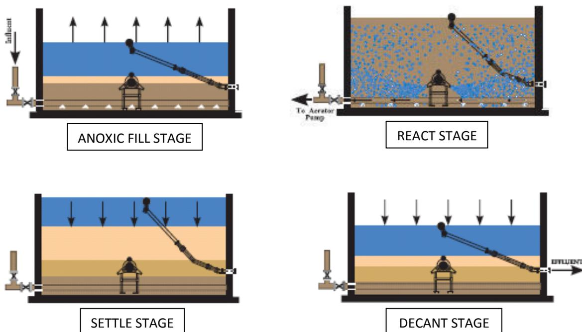
Feed wastewater is treated in a series of steps or processes in the same tank. In the basic form – these are four steps in sequence: (a) Fill (wherein the wastewater is fed in a half-empty basin), (b) React (whereby air is introduced in the basin for a fixed duration), (c) Settle (whereby the MLSS in the tanks are allowed to settle by not allowing any feed or aeration) and (d) Draw (whereby the clear supernatant is withdrawn by a moving weir)
