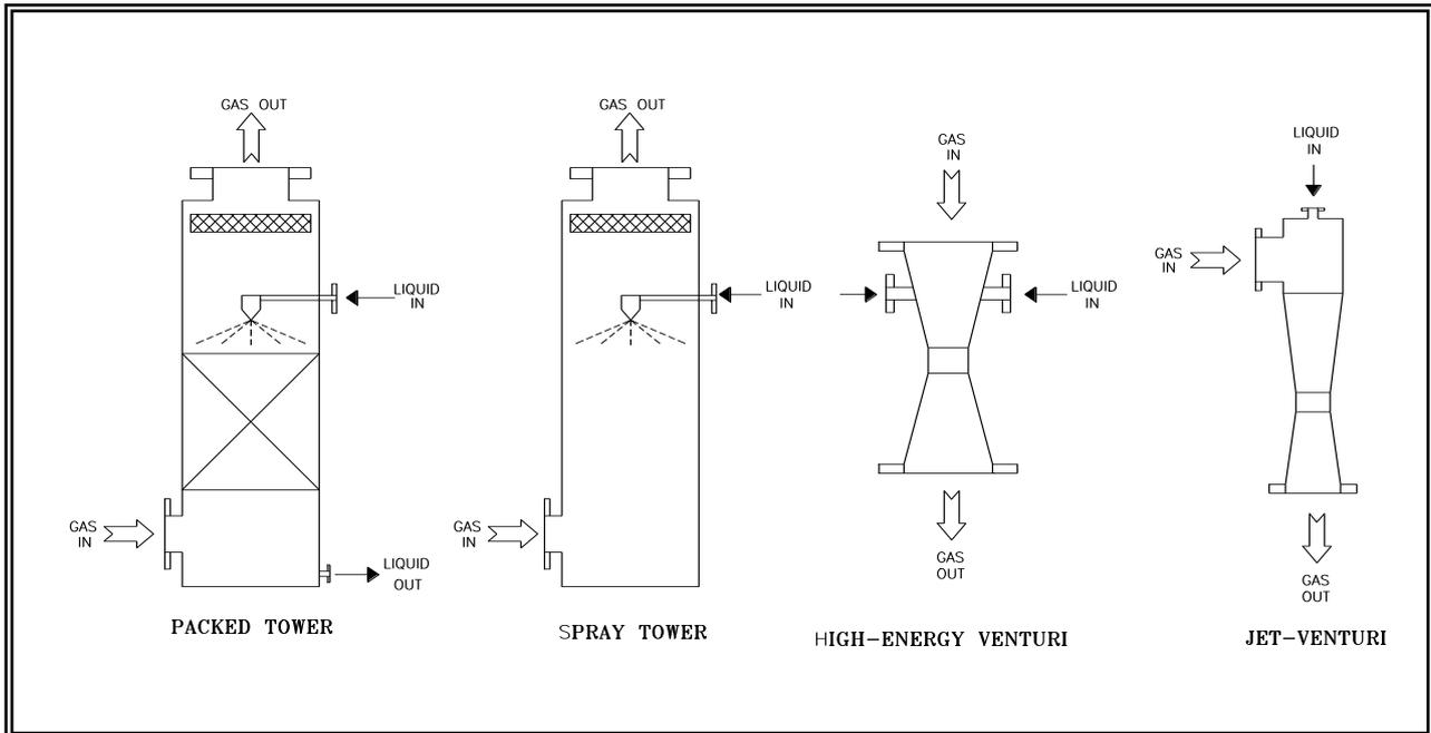
Normally, all Packed Towers for pure gas/mixture scrubbing applications are designed for counter current operation with liquid sprayed on up-flowing gas. Provision of specially designed packings with high specific surface area (surface area per unit volume) gives very high removal efficiencies in practical tower heights. For the same performance, a spray tower system would require 2 –4 times the height or multiple stages.
